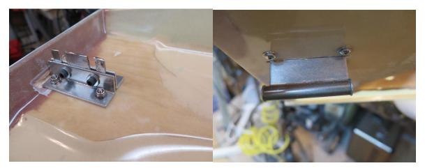
I had to hog out the transom a little bit to clear the strut brackets. After the installs were done and I stripped the boat for paint I floated in some West Systems mixed with West 405 filler and tilted the boat up at an angle to get the epoxy lay in there.
