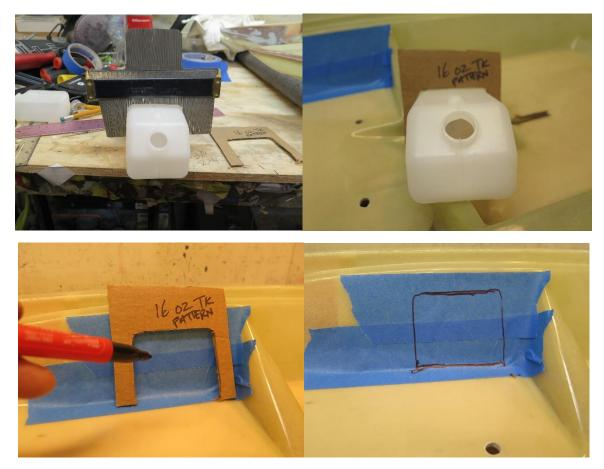
A contour gauge is very helpful in making patterns. Another area where you want undersize the pattern a little bit so that you can gradually remove the least amount of material from the hull. I used the same rotary bits as on the stuffing box.
