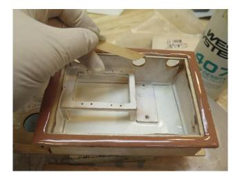
Floating on West with 407 filler. Removing excess that dripped into the radio box lid seat. At this stage I hit the West slightly with a heat gun to put a skin on it and keep it from sagging into places I don't want it to go. This will get a really light block sanding starting with 220 grit and finishing with 1500 grit so the tape sticks really well.
