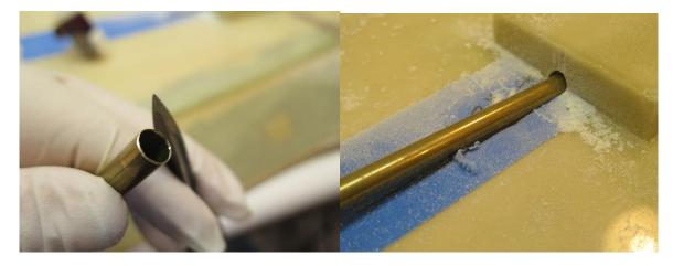
Using a bearing scraper is an easy and fast way remove flash and make the tubing slide easily in and out. If you use a tubing cutter go slow so the tubing is not deformed and reduced in diameter. This part of the process you need to sneak up on and remove as little hull material as possible.
