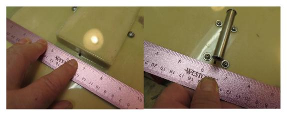
From the data point I measured from the edge of the tunnel to the center of the hole and repeated it to find the center of the strut. If you are doing one of these boats do not go by the indicated measurements because I just butted this scale up against the edge of the tunnel and took the measurement and the scale had about a 1/2" space before the zero mark.
