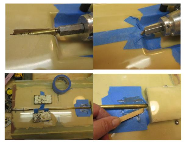
Lay in some West Systems with 405 filler. Wiping up excess epoxy with paper toweling is way easier than sanding it off later and saves a lot of time.
