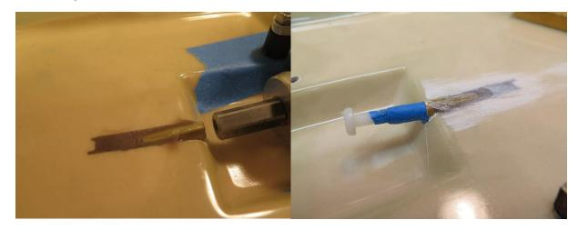
Remove tape and sand flush any epoxy that came through and around where the inner block will go. Pull the motor and mounts and seal off the end of the inner tube with tape and a  $\frac{1}{2}$  screw.
