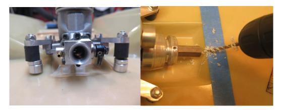
After stacking spacers to get the angle correct and the back of the drive nut centered in the belly pan mark, bore and fasten the motor to the boat. There is just enough space to slide the starter belt under the flywheel and behind the drive nut. Be careful in your fore and aft alignment as well as the side to side. Then bore an 1/8<sup>th</sup> inch hole to data mark the center of the cable location.
