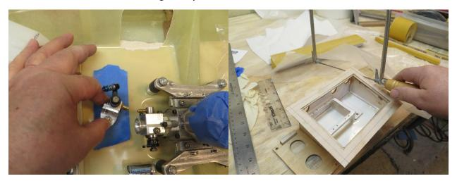
Locating the needle as close as I can to the carb. This way any adjustments take effect almost immediately.
