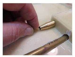
Take the ferrule or another just like it and slide a small hex wrench down the inside edge until you feel it touch the shoulder and transfer that additional distance to the cable and cut the cable and slightly trim the edges where you made the cut.
