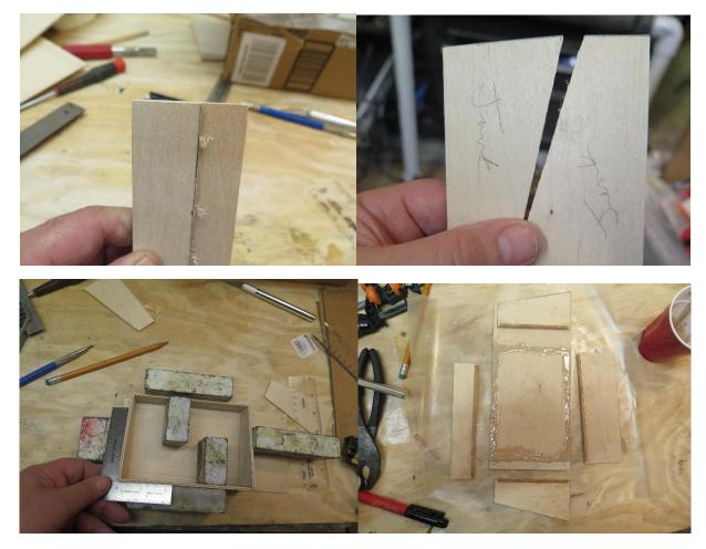
Cutting all the sides out and test fitting them by using weights to hold them in place. The first time I cut out the sides I screwed up two pieces. I always mark my screwups "Junk" and get them off the work bench to avoid compounding the error. I next cut and glued 1/8<sup>th</sup> inch spruce strips to the sides.
