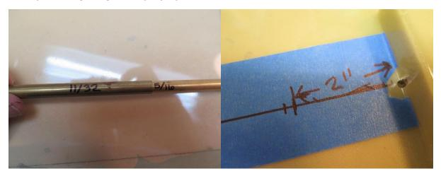
Inner and outer tubes. If you are using a Teflon liner you will have to use different sized tubing. Once the boat is painted and the outer tube reinstalled I will bore an 1/8<sup>th</sup> hole through the inner stuffing tube block and both tubes so I can grease it between runs. Always rough up any tubing in the portions that epoxy will fasten to with 180 grit emery cloth and clean with lacquer thinner.
