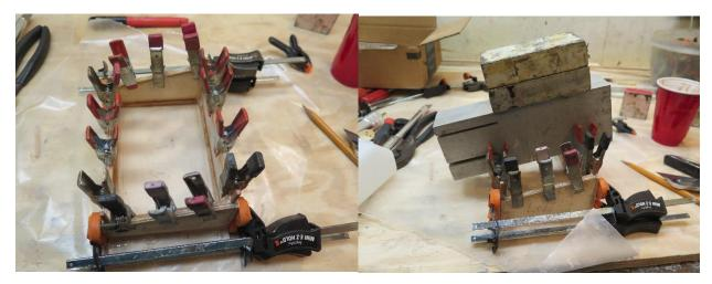
Gluing the box and upper glue strips for the top. Weights help push everything onto the floor.
