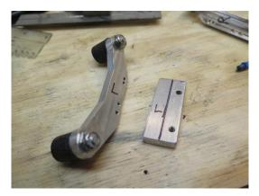
Note labeling to keep your parts straight and aligned. I also cap the isolators with stainless nylock half nuts. Anything that has more than 3 threads exposed gets cut off to save weight.
