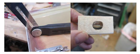
These hulls don't have a ninety-degree transom so I had to make a filler piece out of some really tight grain Maple. I bored out the block to match the hole in the rudder bracket. Note that I roughed up gluing surface with a Dremel wheel.
