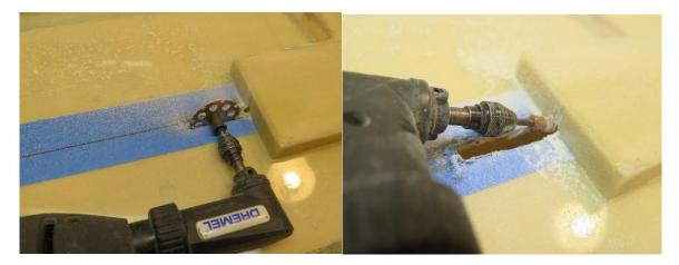
The 90 degree Dremel, tungsten wheels and Robart carbide bits are the bomb for this type of cutting.
