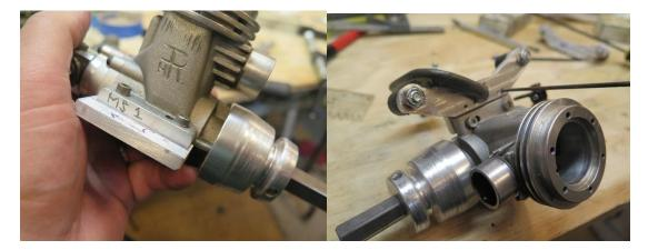
After boring and tapping the transfer block for the motor pattern and attaching it to my set-up motor I clamp the motor mount to the transfer block and using a transfer punch locate where the transfer block will be screwed to the motor mount. A set of transfer punches are invaluable for doing this kind of fabrication work.
