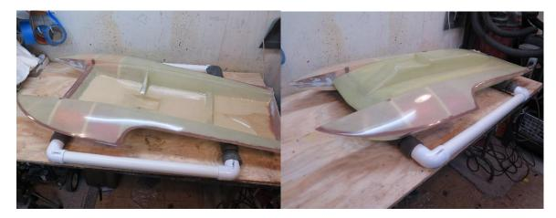
Before starting any work on a fiberglass or carbon fiber hull it needs to get a thorough scrubbing with a little bit of mild detergent dish soap and warm water. I use some of the fine (gray colored) Scotch Brite to assist with getting all the mold release and wax off. Rinse it off and blow it dry with air if you have compressed air. Wait until your wife is not home and give it a rinse in a hot shower.
