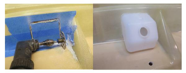
When I reassemble the boat after painting I use RTV silicone and a small piece of carbon fiber angle to hold the tank in place. On these hulls the tank sits just forward of the sponson transom so be careful not to use too long of screws to fasten the turn fin bracket that might pierce the tank.
