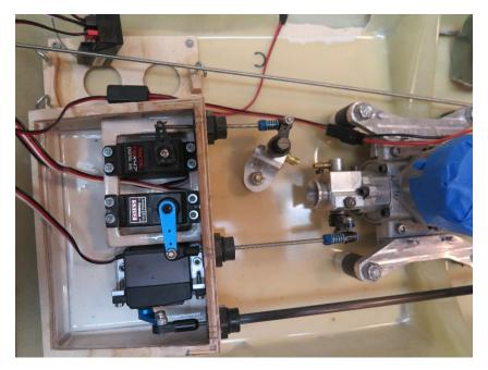
Servo linkages and waterproof boot mounts completed. Make sure there is NEVER any binding in the linkages. It will drain a battery faster than anything and cause a lot of heat that can take down electronic components. The final tasks were to mount the switch and antenna exit.
