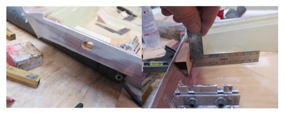
I clamped the rudder into place and cut out the transom where the pushrod runs. Pay attention that the pushrod will clear everything to where the radio box will be installed. Checking that the block will lay at a ninety-degree angle to the bottom. Match up the holes and epoxy in place.
