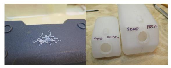
Most experienced builders will tell you an old fuel tank is better than a new one. Here's why. This is the crap that was inside the 16 oz. tank. Before plumbing I inspect the tanks for defects and remove all the flash around the tank necks. Blow them out with air and then slosh around a little denatured alcohol and blow out again. Marking where you want your lines is helpful.
