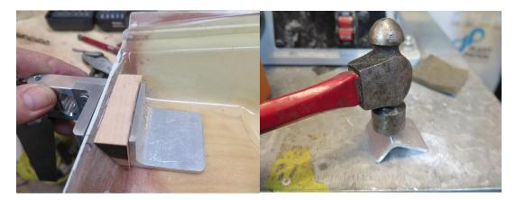
Test fitting a 6061 T6 support bracket. There was a small gap at the top so a little whack with a ballpeen opened up the angle so it sat flush on both contact surfaces. <u>When doing fitment, you never,</u> <u>ever want to build stress into a piece by depending fasteners to pull things in place</u>. Note that a little material has been removed from 90 degree outside edge to accommodate the little epoxy bead at the bottom of the Maple block.
